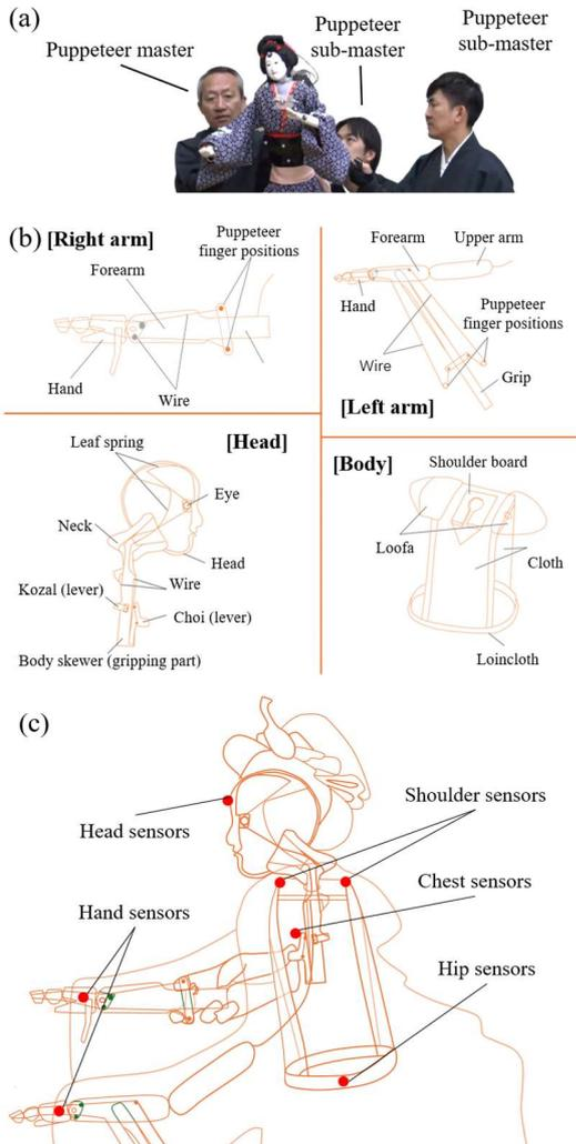
Figure 1. (a) One bunraku puppet. One puppet is operated by one puppeteer master, one left puppeteer, and one foot puppeteer<sup>1</sup>. (b) Structure of a bunraku puppet. The puppet consists of four parts: a right arm, a left arm, a head, and a body. (c) Sensor positions of one bunraku puppet in this experiment (head, left shoulder, right shoulder, left arm, right arm, and chest) [2].
