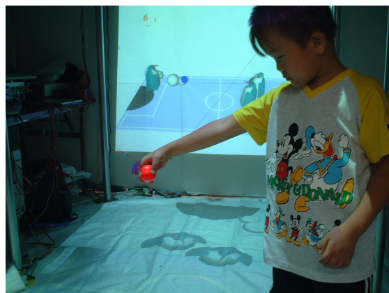
Figure 6. Pictures of Prototype Installation. A player child is grasping a red sphere that is interface of force feedback display. He watches a floor screen. A wall screen is subsidiary.
