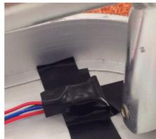
Figure 12: Accelerometers attached to table.
