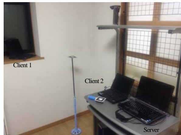
Figure 4. Environment for experiments. A server PC with HMD and two clients PCs with web camera are deployed in a room. The marker information is acquired from the cameras.
