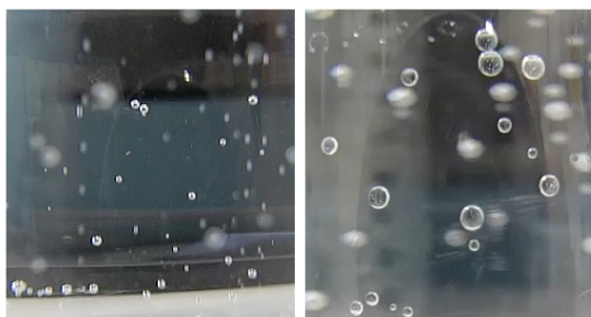
Figure 2: Photographs of the surfaces of containers containing carbonated water. Left: a glass, right: a plastic bottle, taken at the same distance. The sizes of bubbles also differ due to the difference of materials.
