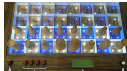
Resignation button Liquid crystal display 16 characters, 2 rows End turn button Promotion buttons From the left: rook, knight, bishop, queen
