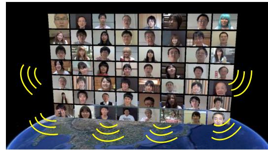
(a) About 25~80 virtual displays are put in a 3DCG space, and each of them plays video clips simultaneously. The system would synthesize sounds of a crowd
