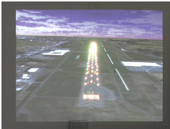
Figure 8: Imitation of a flight simulator scene. The landing runway is lit up using the laser projector.
